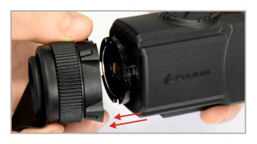
Separate observation eyepiece from the housing.
