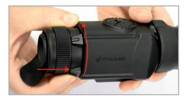
Turn the holding ring counterclockwise with a slight force until stop.
