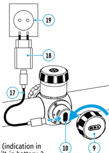
**Attention!** When charging rechargeable batteries with a USB Type-C connector (10) in the riflescope body section, charging priority is given to the built-in battery. When the device is off, both batteries are charged at the same time. When using the device, the external battery is discharged first.
