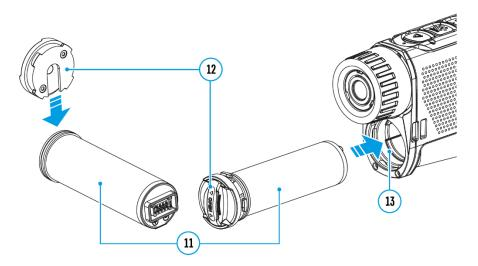
**Attention!** Before installing the battery, make sure that there is an undamaged rubber insulating ring on the battery. The ring is designed to protect your device from moisture getting inside. To replace or purchase a ring, contact your <u>local distributor</u>.
